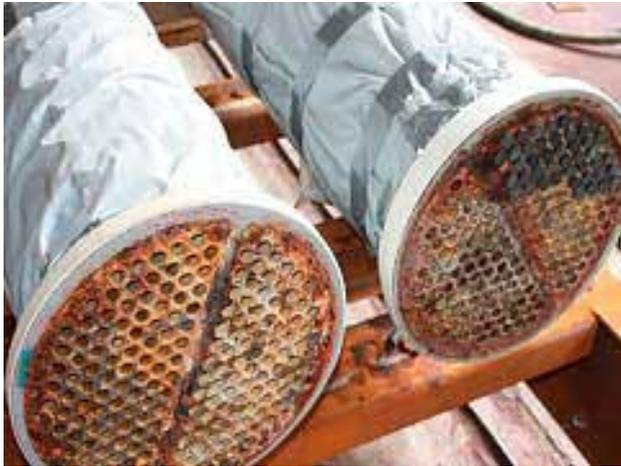
**Cooling water exchanger bundles as received at Curran shop.**
