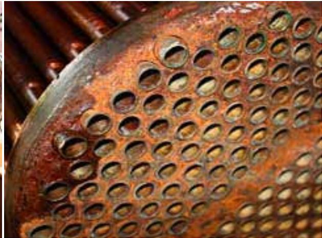
**Close-up of exchanger tube sheet shows evidence of galvanic corrosion attack, coupling of alloy tube and carbon steel tube sheet.**
